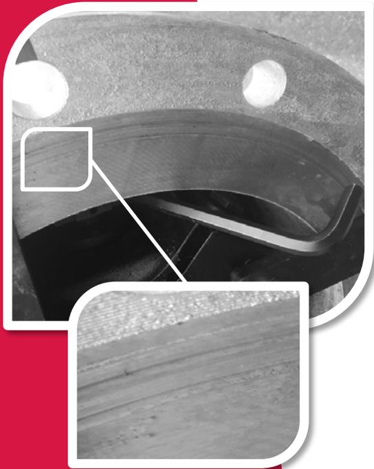
Above: One of the problem flanges showing the rejected surface finish and grooves caused by movement of the machine during operation.
