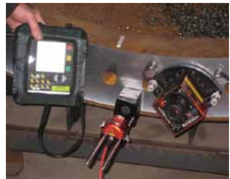
Below: flatness tolerance required 0.30mm with 0.8 – 1.6 \mu\text{m} Ra Finish
