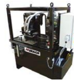
PP4 - 35 Kw Power Pack Diesel engine silent type, complete with 12 volt control variable delivery axial piston pump with constant pressure control, variable output flow, 0 to 80 L.P.M up to 160 bar
