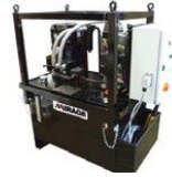
PP4 - 35 Kw Power Pack Diesel engine silent type, complete with 12 volt control variable delivery axial piston pump with constant pressure control, variable output flow, 0 to 80 L.P.M up to 160 bar
