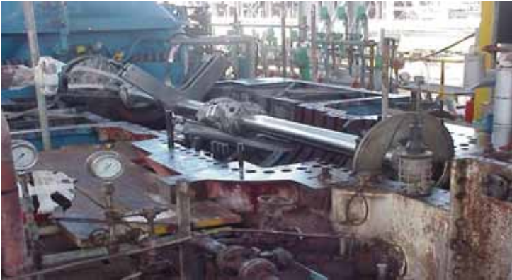
(Above) Machine being loaded into the GE Turbine and the (left) surface finish achieved
