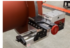
MM1000i-22 Heat Exchanger Back Facing Kit
