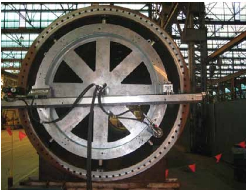
Left: the WP4300 mounted into a tower flange
